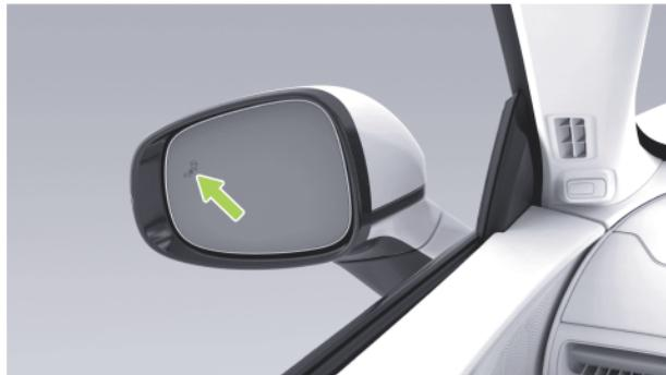
Vehicle in D, vehicle speed greater than 10 km/h, if vehicle is in blind area, or fast approaching vehicle is behind blind area, The warning light in the corresponding exterior mirror is permanently lit, and the warning light in the exterior mirror changes to flash to alert you if the opposite traffic light or turn signal is turned on.
