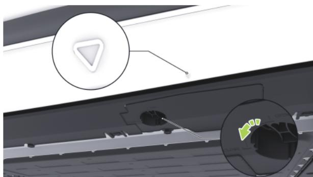
The position of the vehicle lifting point is confirmed by the arrows in the lower door trim. The trim panel is mounted under the lifting points and can be removed by turning the knob on the trim counter-clockwise. Remove the trim from the lifting points before lifting the vehicle using a jack.
