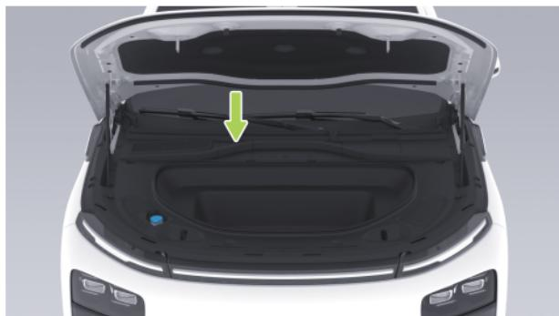
1. Open the front compartment and remove the front compartment access cover.
