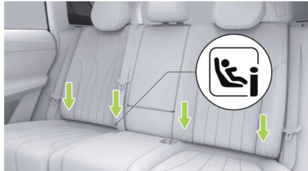
The ISOFIX anchor points are located between the rear seat back and the seat cushion, and are stamped with an ISOFIX logo above the anchor points.
