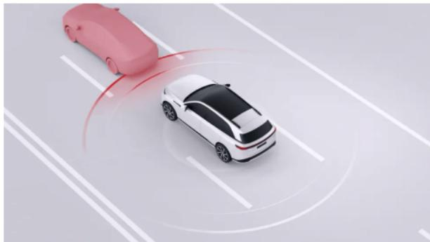
Forward Collision Warning includes Forward Collision Warning (FCW) and Autonomous Emergency Braking (AEB) to reduce the risk of a collision or reduce the speed of a collision and improve road safety.
