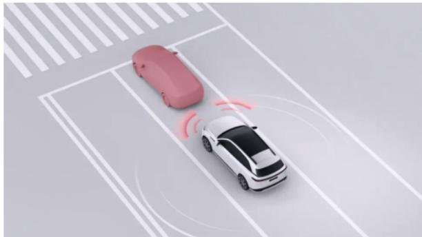
**Drive-away avoidance** When the vehicle is moving away, an obstacle is detected in the direction of travel and the driver presses the accelerator pedal too quickly, limiting the vehicle's dynamic response. Avoid collisions with obstacles caused by electric vehicles accelerating too fast.
