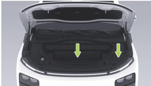
1. Using a suitable tool, remove the front compartment trim panel and the storage box, i.e. the visible coolant reservoir.
