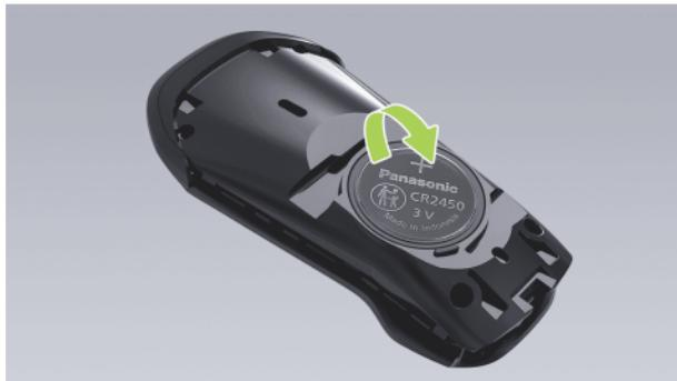
4. Remove the key battery. Battery model: CR2450.
