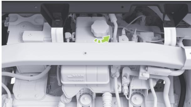
2. Unscrew the reservoir cap and top up the coolant.
