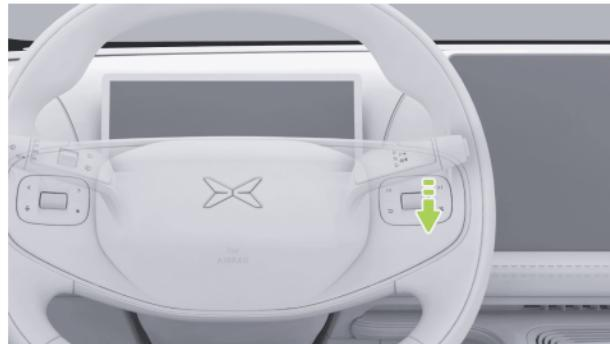
The LCC is activated by pushing the selector fully down 2 times and the SR screen light up, accompanied by a voice prompt.
