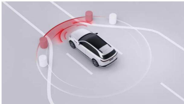
The vehicle is in D, vehicle speed is less than 15 km/h and an obstruction is detected on the front and rear sides of the vehicle, the vehicle will
