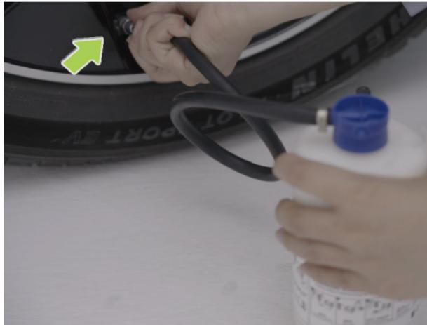
4. Screw one end of the tire repair glue joint into the tire valve and tighten. Be careful not to turn the tire repair glue pot upside down.
