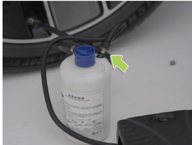
5. Connect and tighten the additional tire repair glue pipe to the charge pump and connect the charge pump power cable to a 12V power supply in the vehicle storage box.
