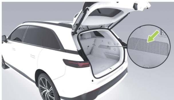
1. Open the rear trunk and use a suitable tool to open the rear trunk service cover.
