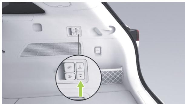
Pressing the suspension raise or lower switch in the trunk allows the trunk height to be adjusted for easy loading and unloading.
