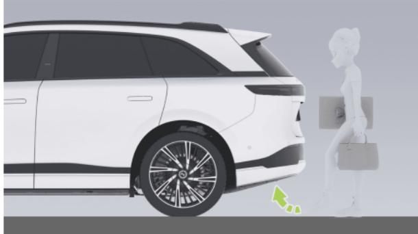
If the remote key is present in the trunk access area, the trunk can be unlocked and opened or closed by foot movement.
