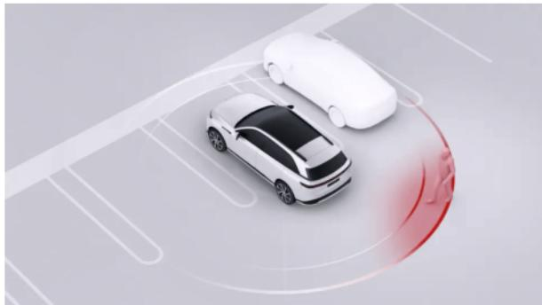
When reversing, the Driving Aids system detects if a standing or transverse pedestrian behind is within the range of the vehicle and may collide with the vehicle. In this case, the reverse collision prevention system will assist the driver with the brakes to prevent or reduce impact damage. The system also provides feedback to road traffic participants outside the vehicle via the brake lights, reminding them to avoid.
