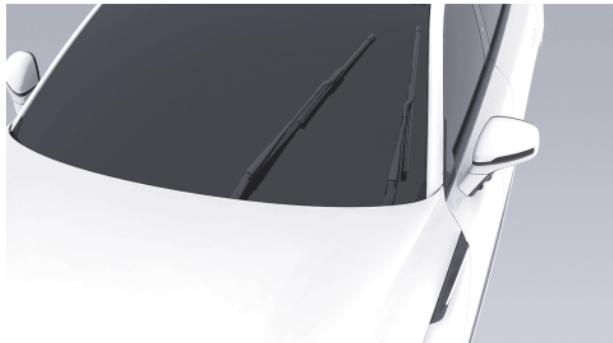
With the vehicle in P position, leave the wipers off. In the central control screen “ **Vehicle**” interface, Open “**Front/Rear Wiper Maintenance Mode**”, The wiper arms will operate to the service position and return automatically when the wiper service mode is switched off.
