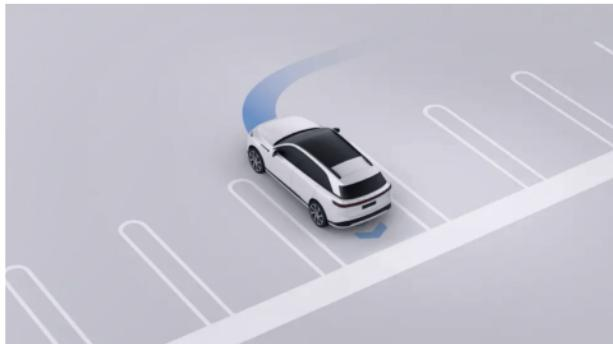
The APA assists the driver in and out of vertical, parallel and diagonal parking spaces for both wired and wireless boxes and supports the following activation methods:
