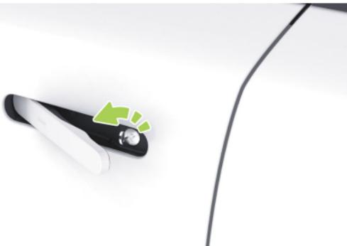
When the vehicle is de-energized, press the flush door handle forward to pull the door handle, fully insert the mechanical key into the locking hole and turn the door counter-clockwise to unlock. Pull the door handle to open the door.
