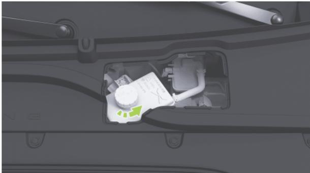
3. Unscrew and remove the reservoir cap.
