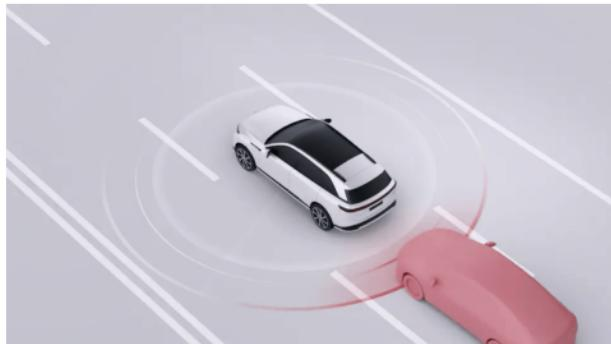
When driving, the RCW detects and alerts you to a collision hazard behind the vehicle.
