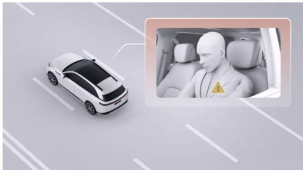
The DSM monitors the driver's status while the vehicle is moving and provides warnings if the driver shows a state of distraction or fatigue.
