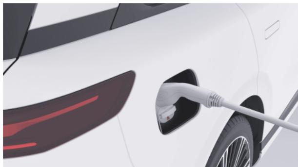
5. Insert the charge gun vertically into the charging port and hear a click to indicate that the charge gun is in place.
