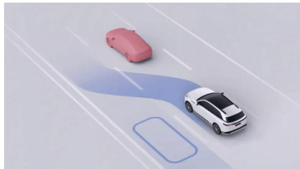
When LCC is active, the traffic lights are switched on and the ALC can assist the driver in changing lanes.
