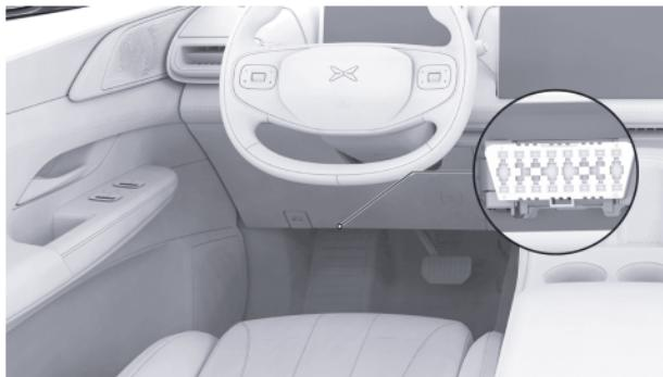
The OBD interface for reading the electronic VIN code is located on the lower left of the instrument panel and data such as the electronic VIN code and vehicle status information can be read via the factory diagnostic tool or the factory official approved diagnostic equipment.
