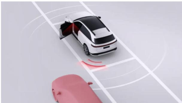
The DOW alerts the occupants of the vehicle when there is a risk of collision when the door is opened.
