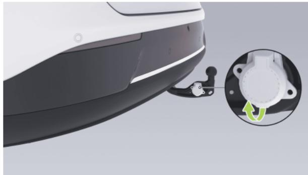
The electrical connection connector is mounted on the towbar and extends with the towbar when the towbar switch is activated on the center screen. Once the protective cover is open, it is ready for use.
