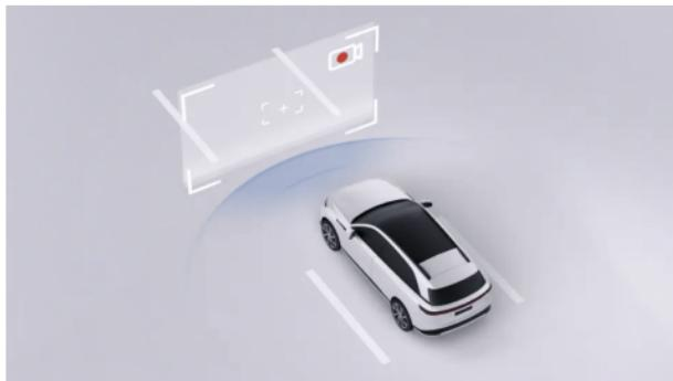
The Drive Recording feature enables video recording of the vehicle while driving and stores the video on a USB stick. Video files can be used to view past information when the user needs it, or used to assist in evidence collection in the event of an accident.
