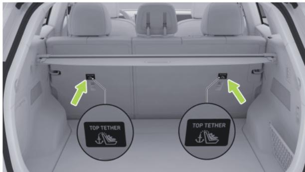
The upper anchor point is located behind the rear seat backrest on both sides.
