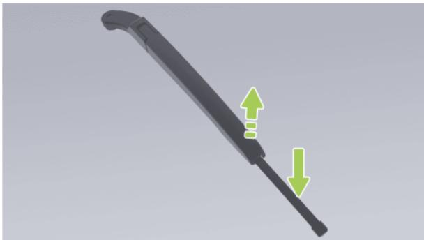
2. Remove the wiper blades by pressing and holding the wiper blades and pulling the wiper arms upwards along the wiper arms and blade connections.
